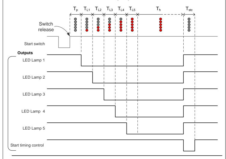
Timings shown are configurable from 0 to 25.5S in 100mS intervals  $T_h$  can be fixed or random delay
